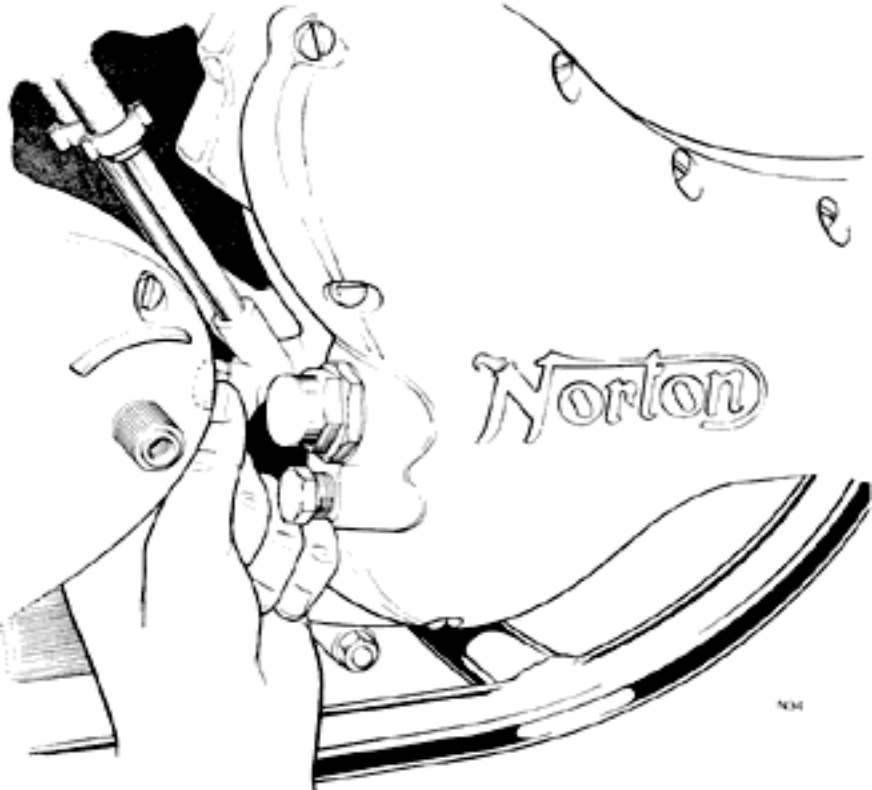
Fig. F1 Removing oil junction block securing bolt
