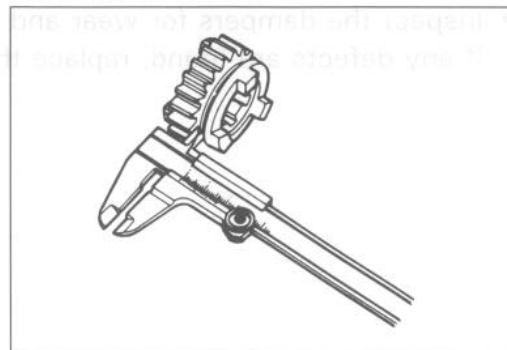
Checking groove width
